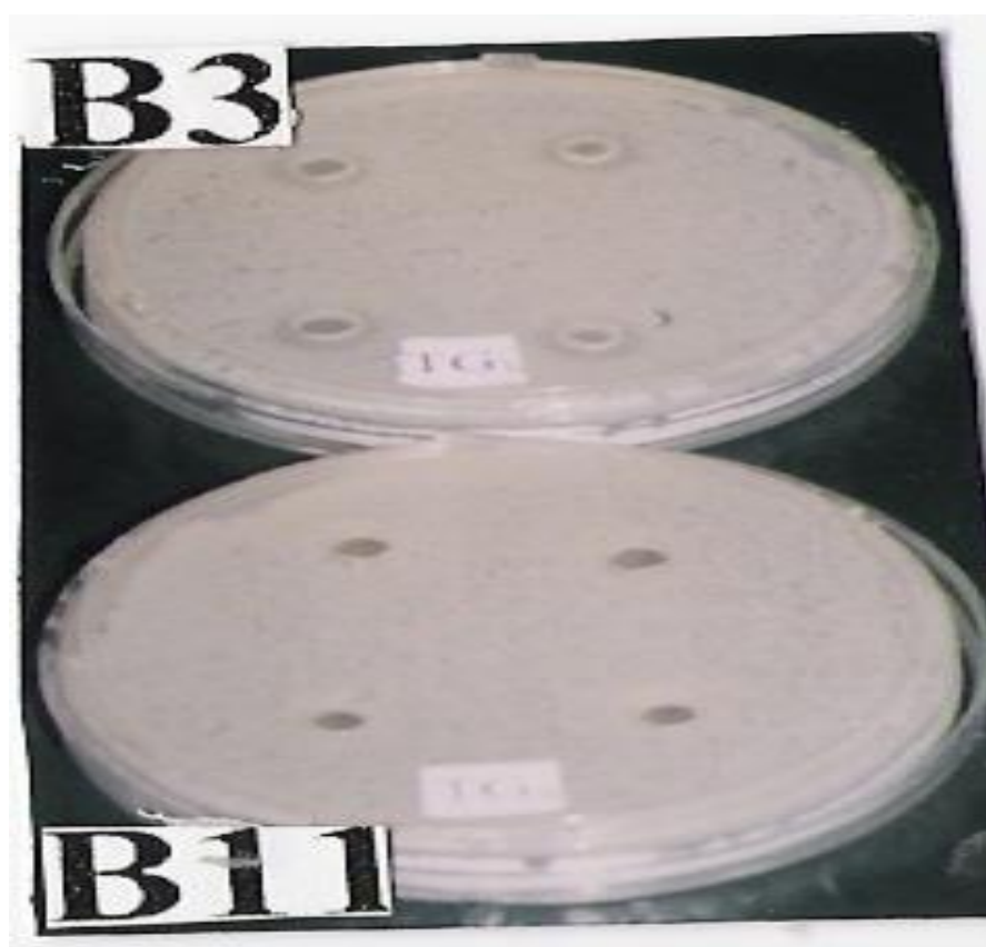
Figure 4.1 Illustration of inhibition zones in 80% hexane: 20% dichloromethane (B 3 ) and 100% water (B 11 ) biotest solutions
