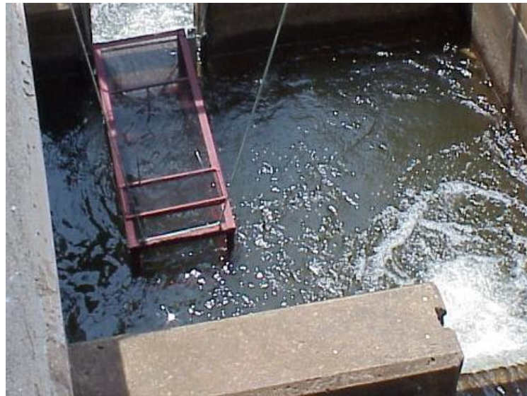
Figure 8.2: The placement of the trapping cage in the notch in the baffle of the fishway at Xikundu.
