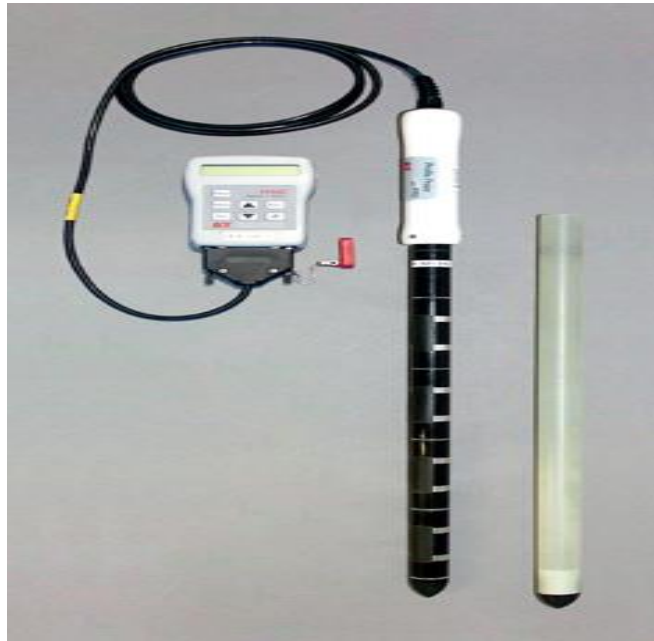
Figure 3.2. HH2 moisture meter and PR2 profile probe for soil moisture measurement.
