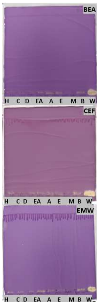
Figure 4.1: DPPH free radical scavenging activity evaluation of Cassia petersiana extracts from preliminary extraction. The yellow colour behind the purple background of DPPH indicates antioxidant activity.
