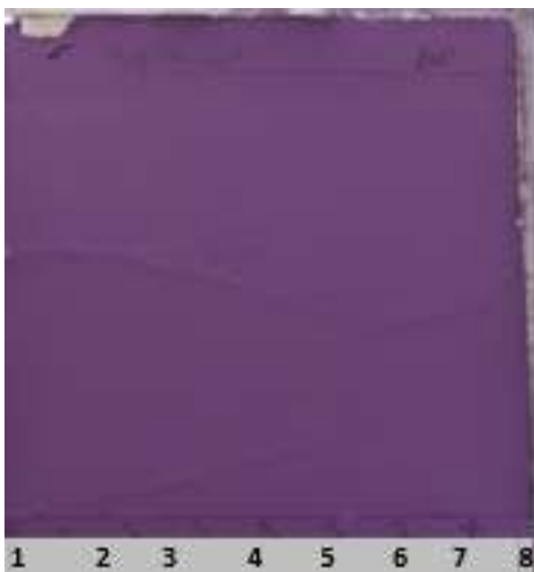
Figure 7.8: TLC-DPPH assay for antioxidant activity of the combined fractions from column chromatography. Antioxidant activity, which is indicated by the yellow bands behind the purple background, was not observed.
