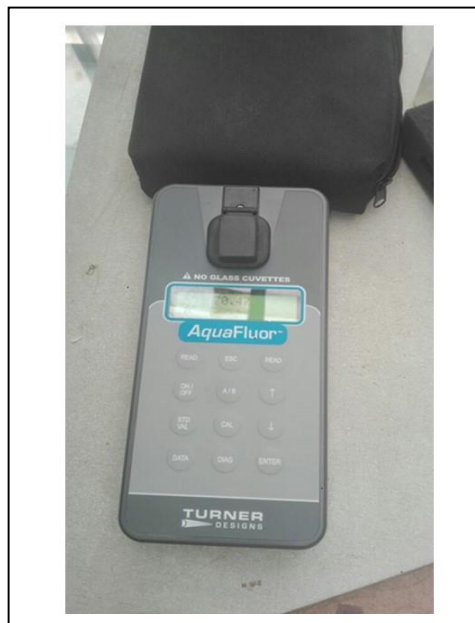
Figure 2.5: A handheld fluorometer (AquaFluoro®) used to measure chlorophyll-a concentrations
