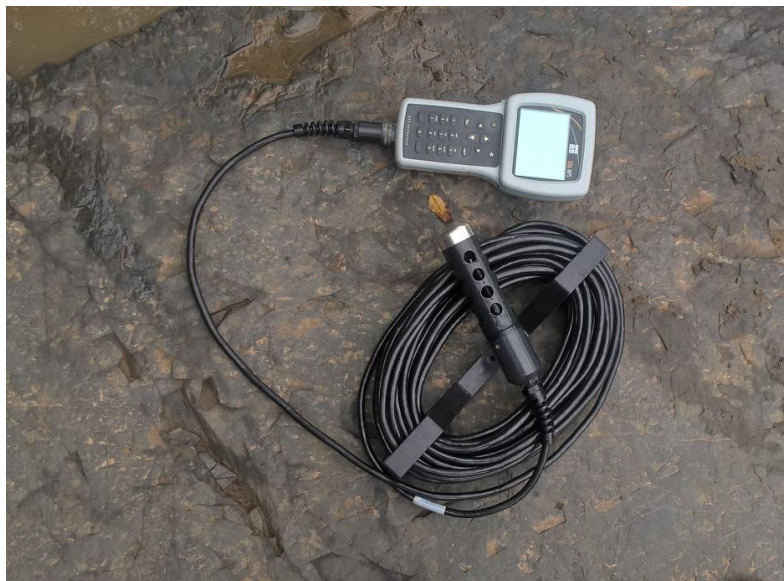
Figure 3.1 YSI meter used to measure system variables at Loskop and Flag Boshielo dams during 2014 surveys.
